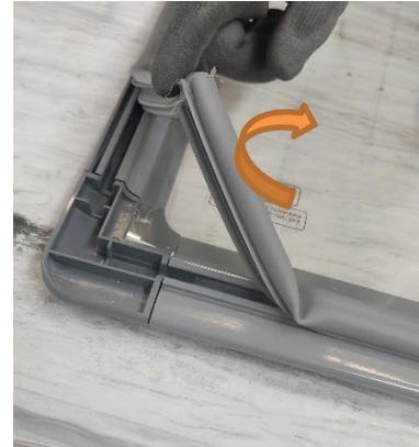
*Fig 16.b. Apply silicone to the edges of the lid profile.*
