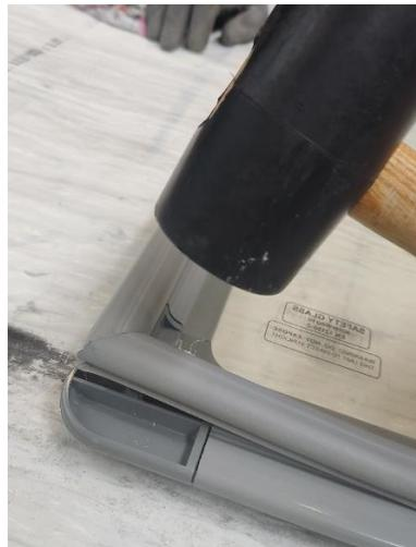
*Fig 16.d. Use the rubber mallet to adjust the seal on the lid profile gap.*
