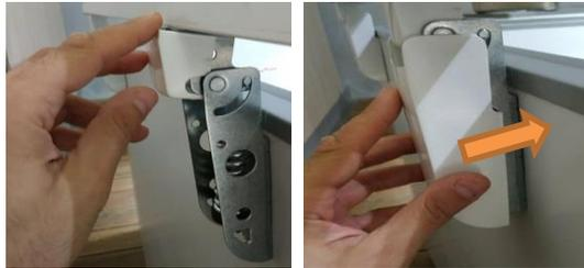
Fig 9. Hinge cover placement
