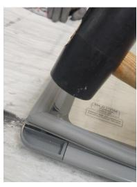
Fig 16.d. Use the rubber mallet to adjust the seal on the lid profile gap.
