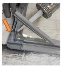
Fig 16.c. Insert the new seal in the seat of the lid profile.
