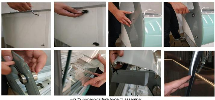
Fig 13.Hyperstructure (type 1) assembly
